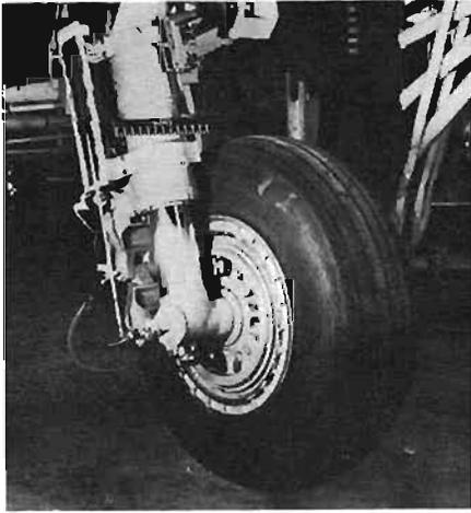
Test aircraft tire: 44x13 Type VII, rib tread.
