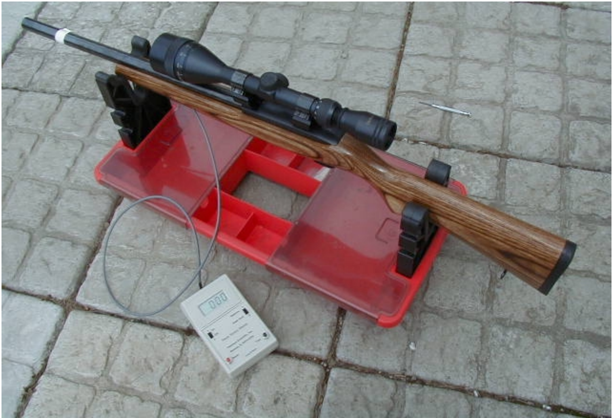
Figure 3: Modified Ruger 10/22T with peak strain meter
