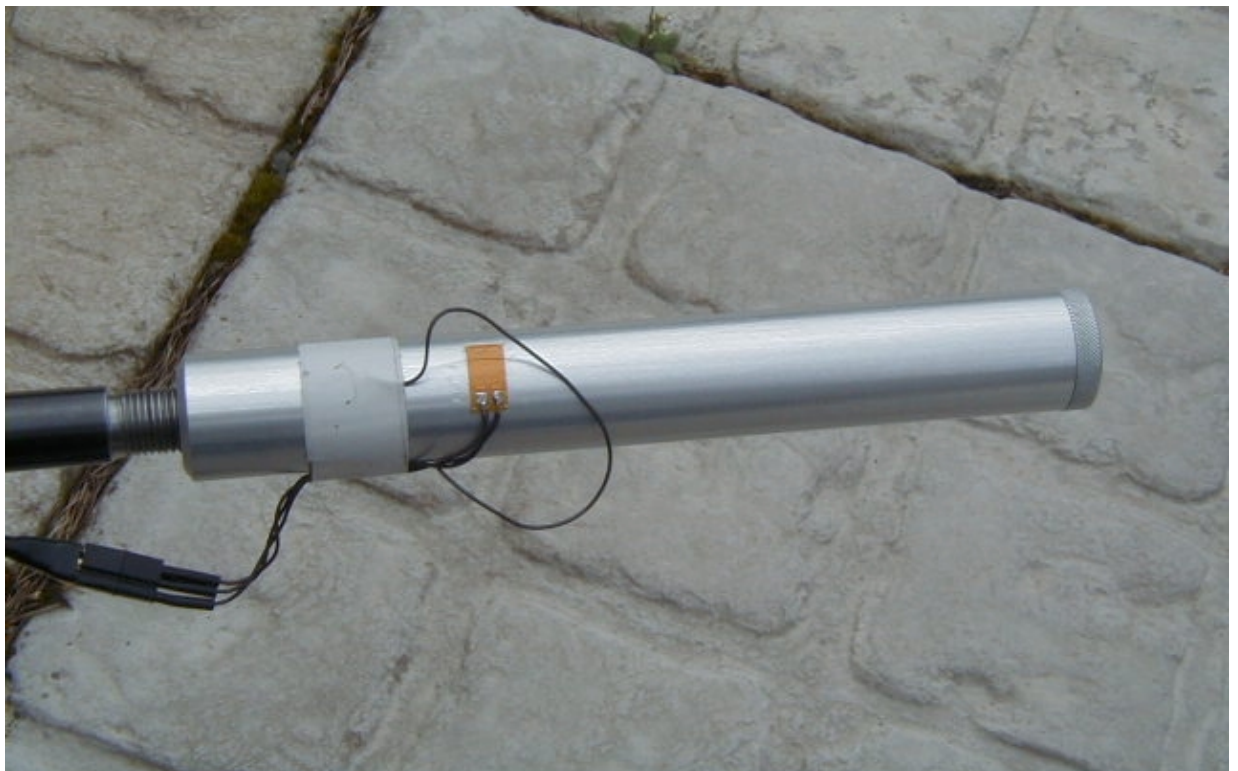
Figure 8: Strain gauge on detachable aluminium sound moderator
