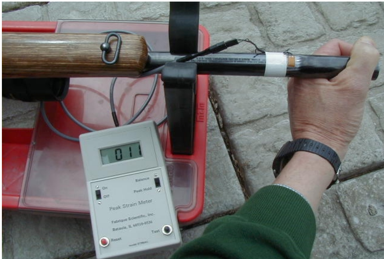
Figure 5: Strain applied by hand to check strain gauge and meter operation
