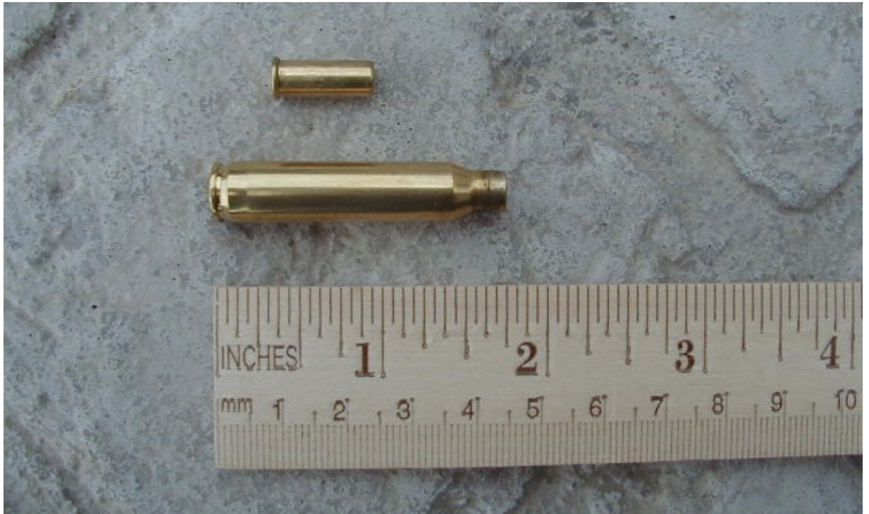
Figure 7: Comparison of .22 LR rim-fire and 223 Rem. centre-fire cartridge cases
